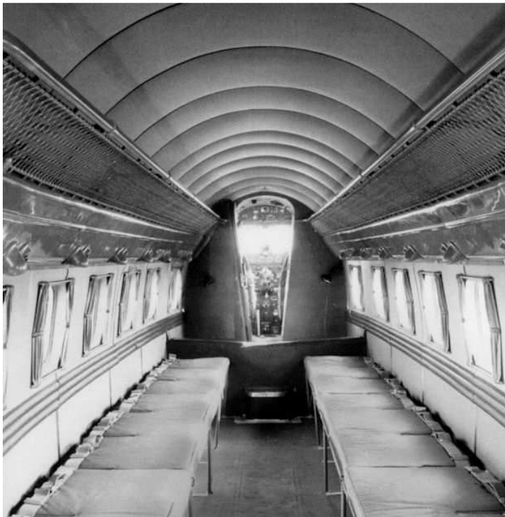
Photo 3: Factory photograph of the already spartan original interior of the L18. The racks for luggage and the parachutist seats along the fuselage were completely removed by the Technical Service at Andir (Lockheed photograph, via G.J. Casius).
