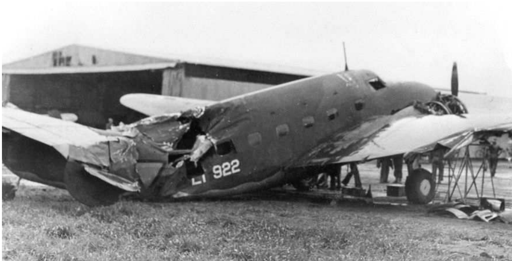
Photo 2: Wreck of the LT922 at Archerfield late February 1942. ML and USAAF personnel are busy taking off the engines to transfer these to aircraft LT919 (Alan Bovelt collection, via Gerard Casius and Gordon Birkett).
