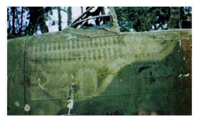
Picture 1: The wreck of the ex MLD Boston AL907/A28-8, recovered in Goodenough Island in 1987. On the nose the number 240, the 240<sup>th</sup> and last aircraft of the original French order, applied for publicity reasons by Douglas, is still visible (RAAF Museum, through Charles Kranenburg).
